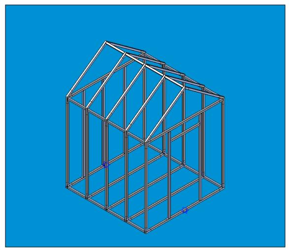
ABOVE DISPLAY IS AN 8X8 PORTABLE STEEL SHED FRAME WITH FLOOR STRUTS ON
